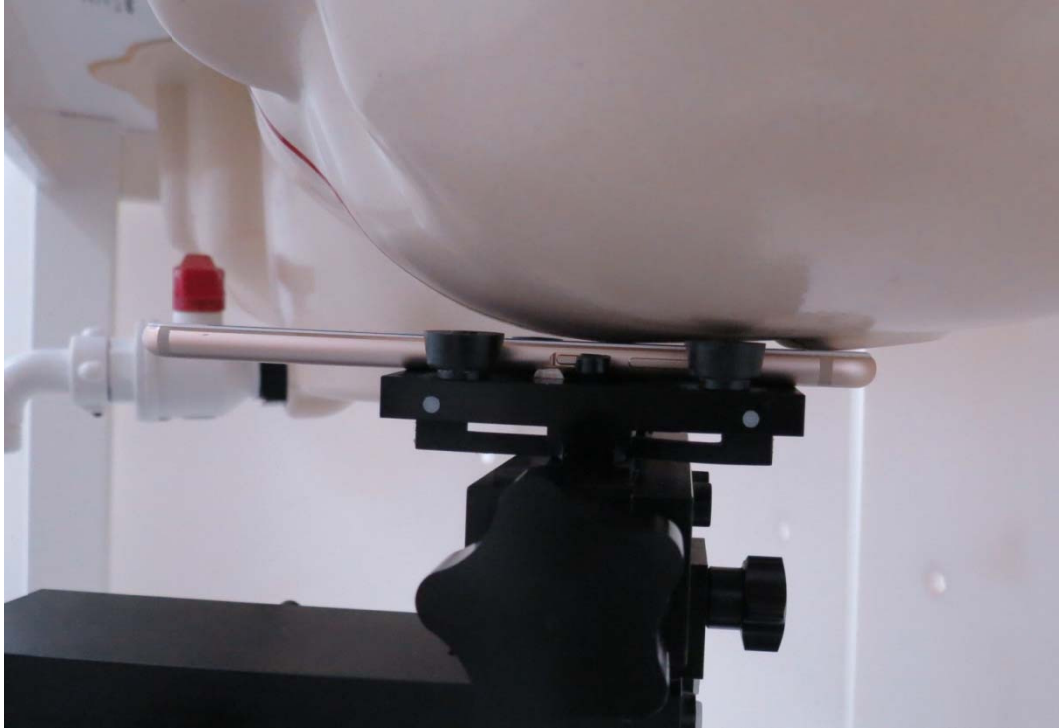
Picture 2: Left Hand Touch Cheek Position
