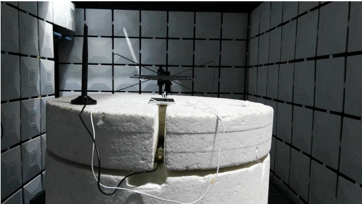
Radiated Spurious Emission (3GHz to 18GHz)
