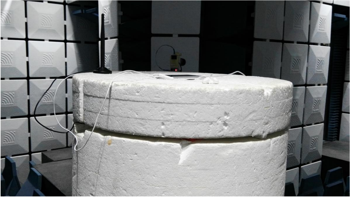
Radiated Spurious Emission (18GHz to26.5GHz)
