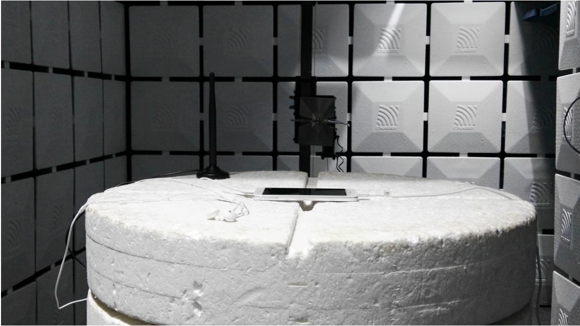
Radiated Spurious Emission (below 3GHz)
