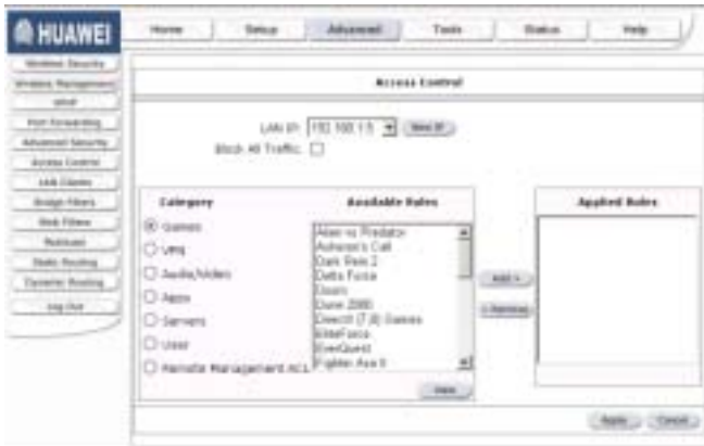
Figure 3-32 Access Control menu
