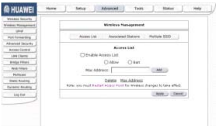
Figure 3-38 Access Control based on the MAC address
