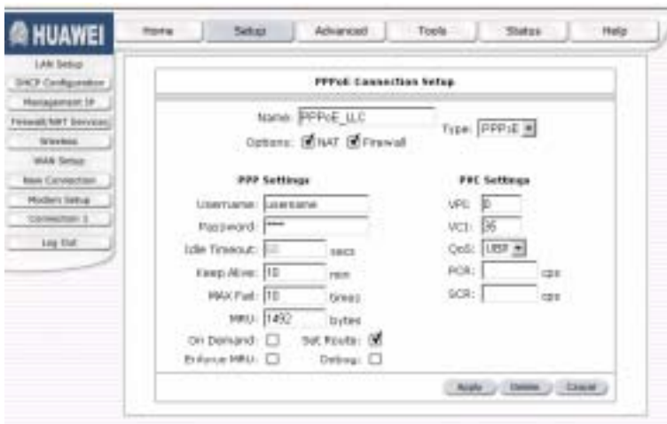
Figure 3-14 Setup – Configure Connection 1 for PPPoE
