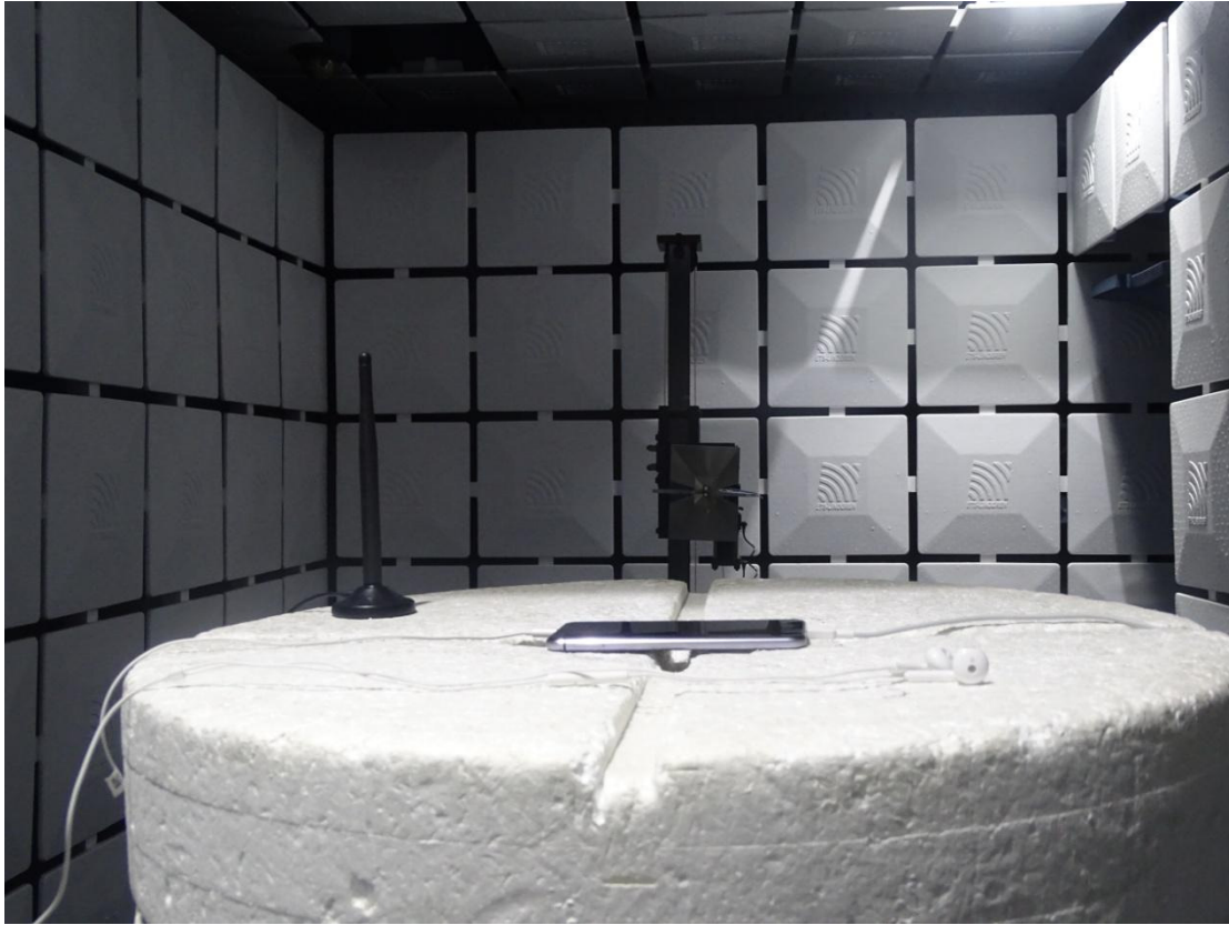
Radiated Spurious Emission (3GHz to18GHz)
