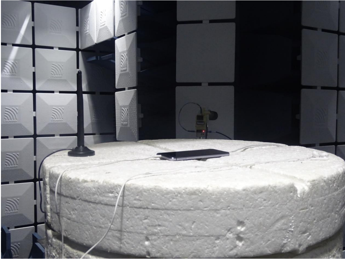
Radiated Spurious Emission (18GHz to26.5GHz)
