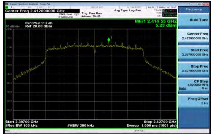
802.11n_HT20 Band Edge Limit Test Data CH-High
