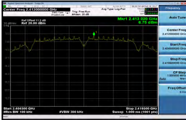
802.11b Band Edge Limit Test Data CH-High
