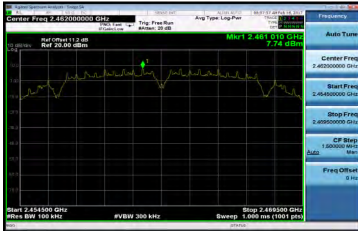
802.11g Band Edge Limit Test Data CH-Low
