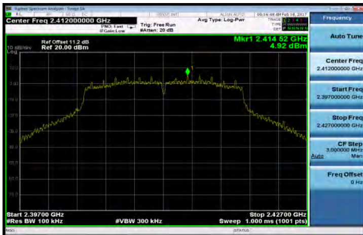
802.11g Band Edge Limit Test Data CH-Low
