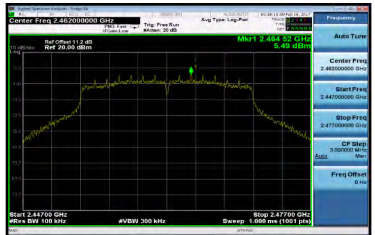
802.11n_HT20 Band Edge Limit Test Data CH-High
