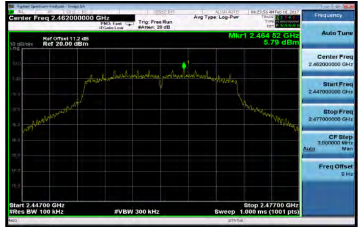
802.11n_HT20 Band Edge Limit Test Data CH-Low
