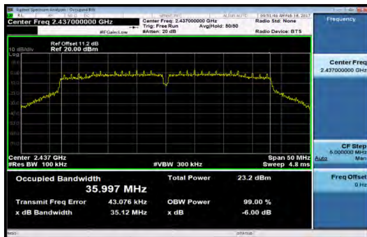
6dB Band Width Test Data CH-High
