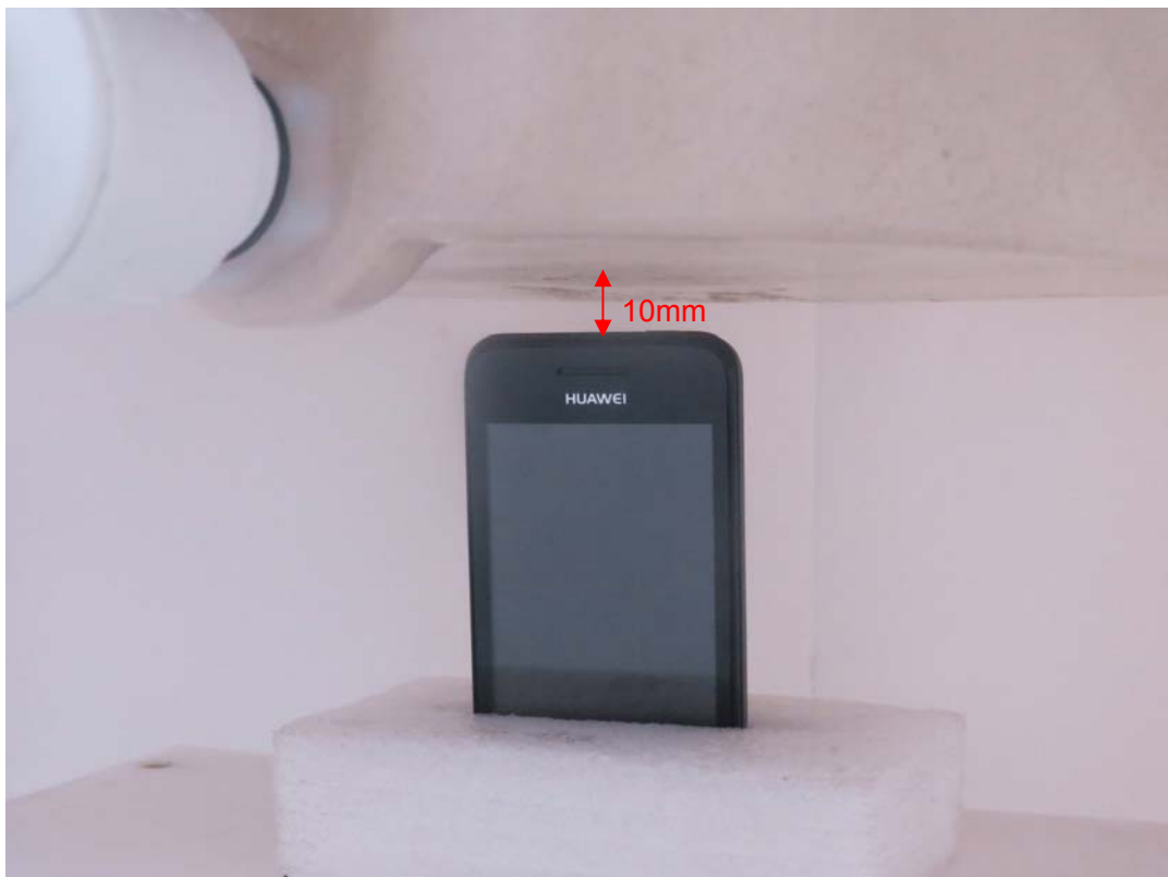
Picture 17: Top Edge, the distance from handset to the bottom of the Phantom is 10mm (Original)
