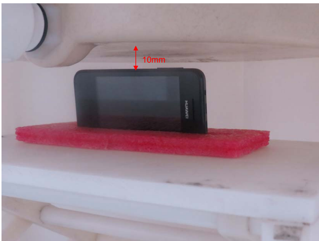
Picture 15: Left Edge, the distance from handset to the bottom of the Phantom is 10mm (Original)
