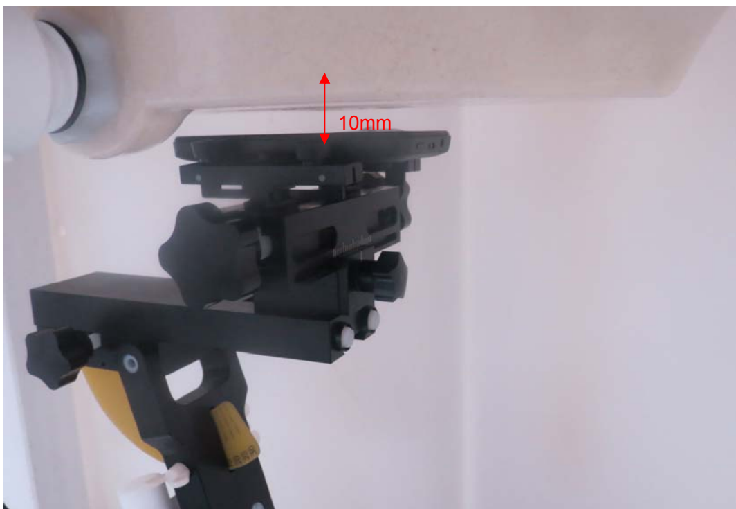
Picture 14: Front Side, the distance from handset to the bottom of the Phantom is 10mm (Original)
