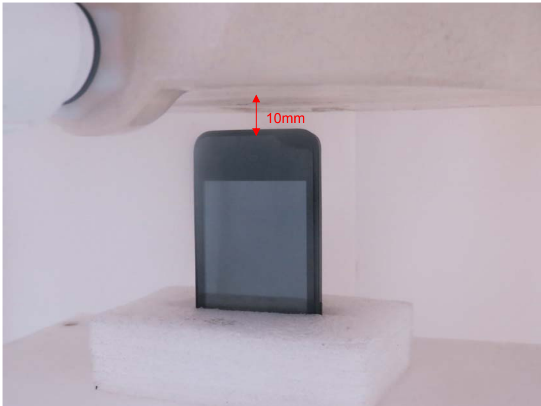
Picture 18: Bottom Edge, the distance from handset to the bottom of the Phantom is 10mm(Original)
