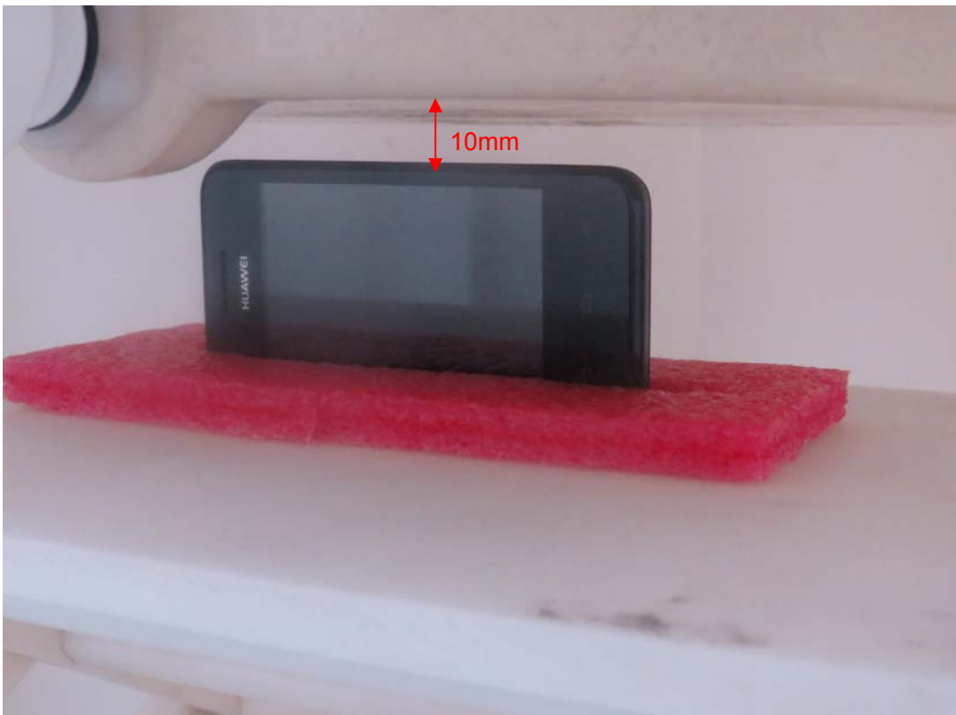
Picture : Right Edge, the distance from handset to the bottom of the Phantom is 10mm
