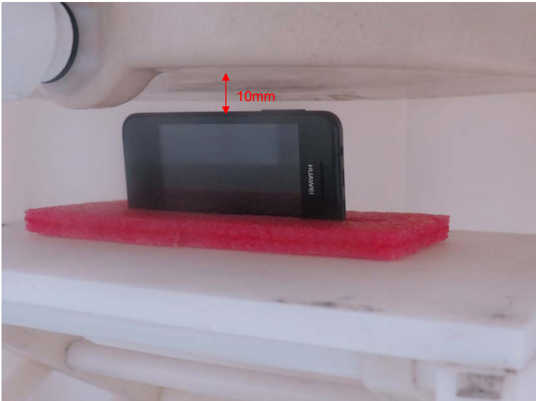
Picture : Left Edge, the distance from handset to the bottom of the Phantom is 10mm
