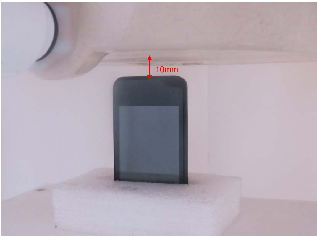
Picture : Bottom Edge, the distance from handset to the bottom of the Phantom is 10mm
