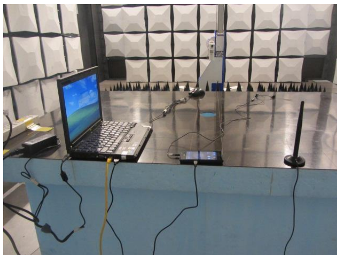
Radiated Spurious Emission (above 18GHz)
