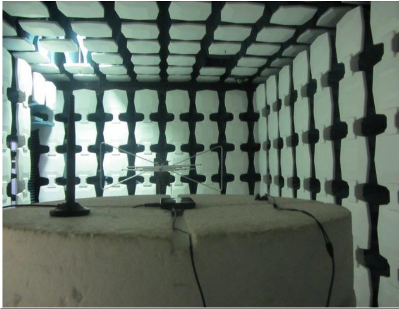
Radiated Spurious Emission (below 3GHz)
