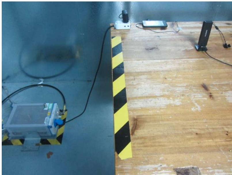
Conducted Emissions for AC Ports
