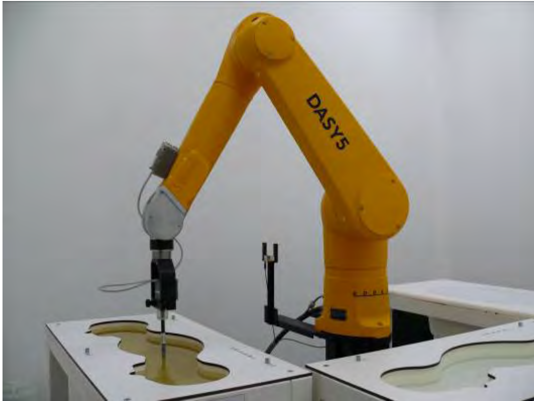
Picture 1: Specific Absorption Rate Test Layout
