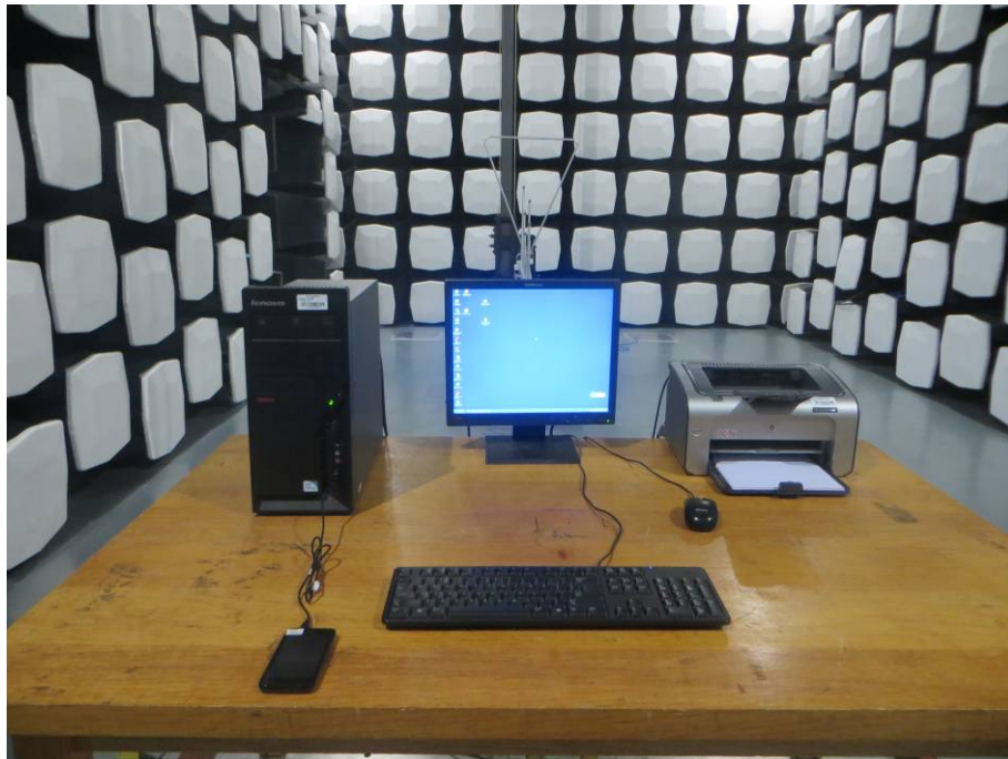
1. Radiated Emissions (Part 15B PC mode) (below 1GHz)
