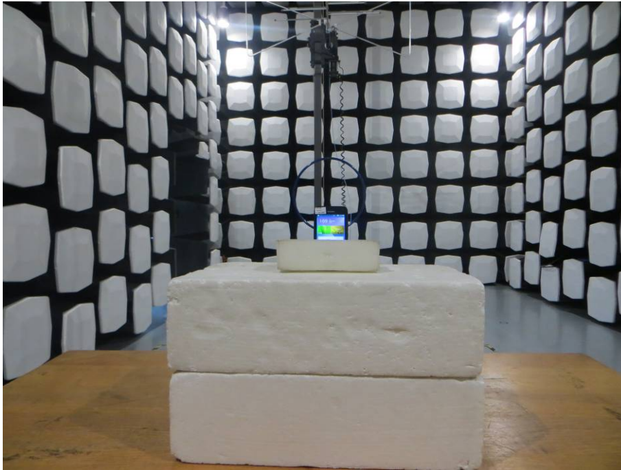
5. Radiated Emissions (Part 15C) (below 30MHz)
