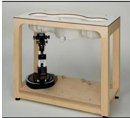
Picture C.10: SAM Twin Phantom
