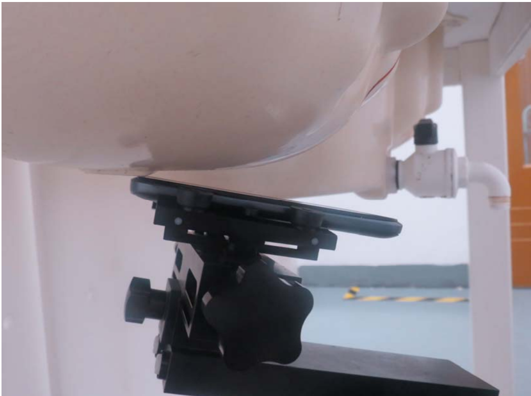
Picture 12: Right Hand Tilt 15 Degree Position
