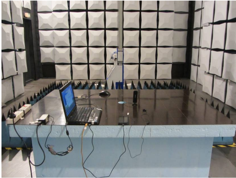
Radiated Spurious Emission (above 18GHz)
