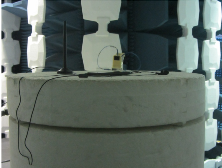
Radiated Spurious Emission (18GHz to26.5GHz)
