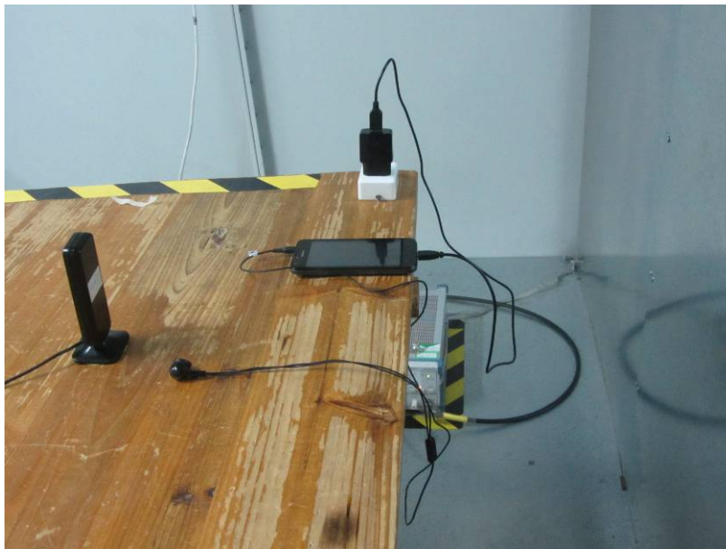
Conducted Emissions for AC Ports
