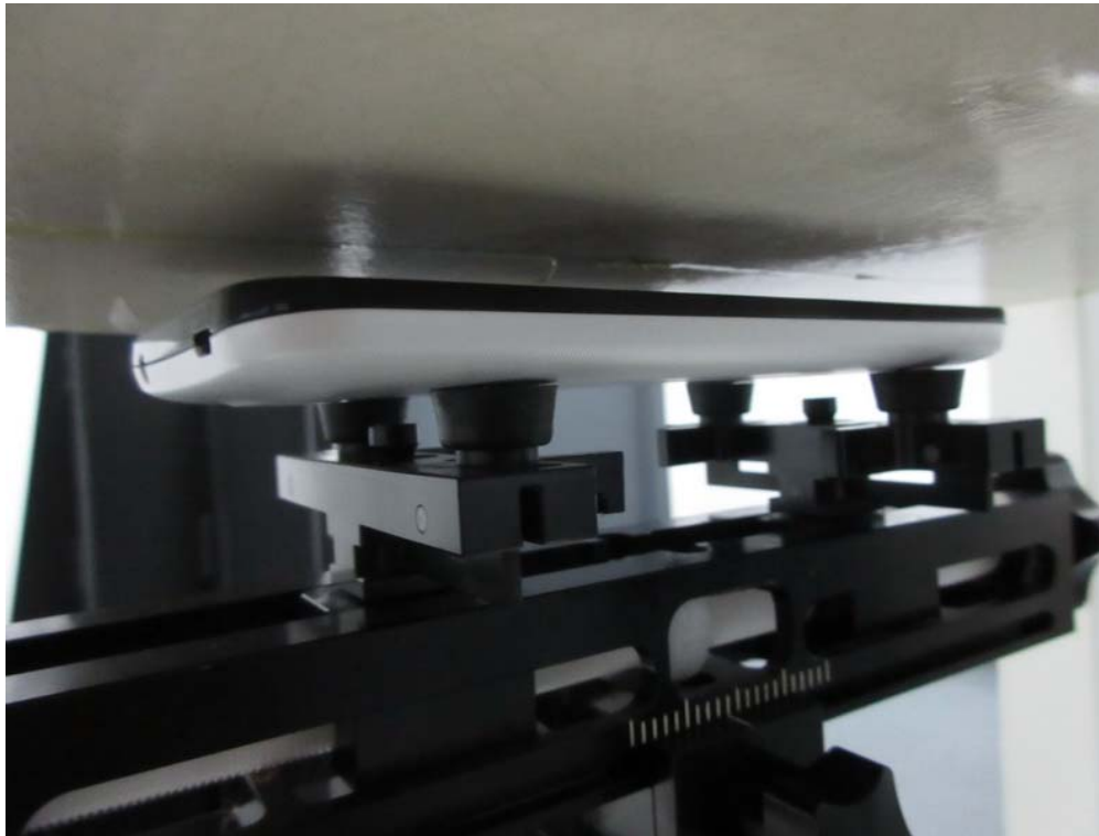
Test Position Front 10mm
