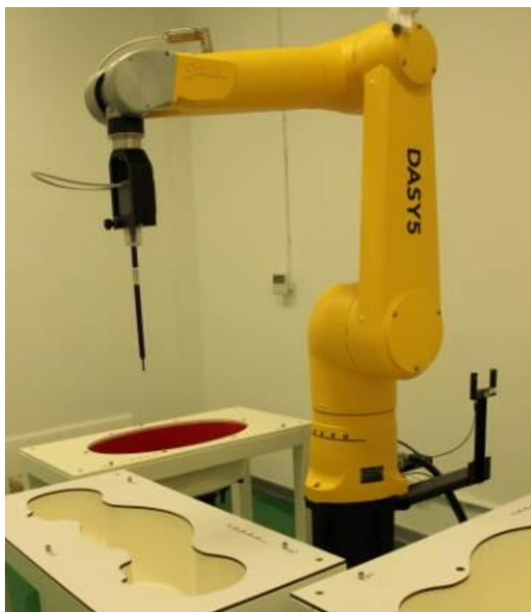
Picture D.6 DSY5 system Set-up
