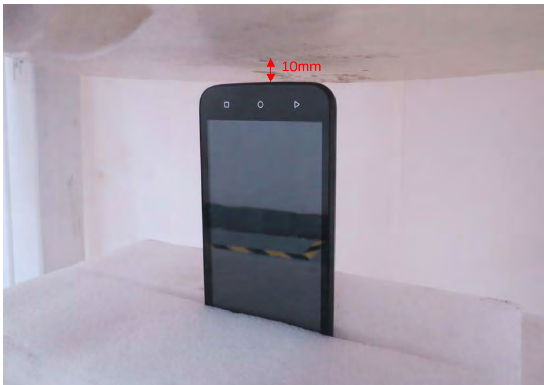
Picture 18: Bottom Edge, the distance from handset to the bottom of the Phantom is 10mm
