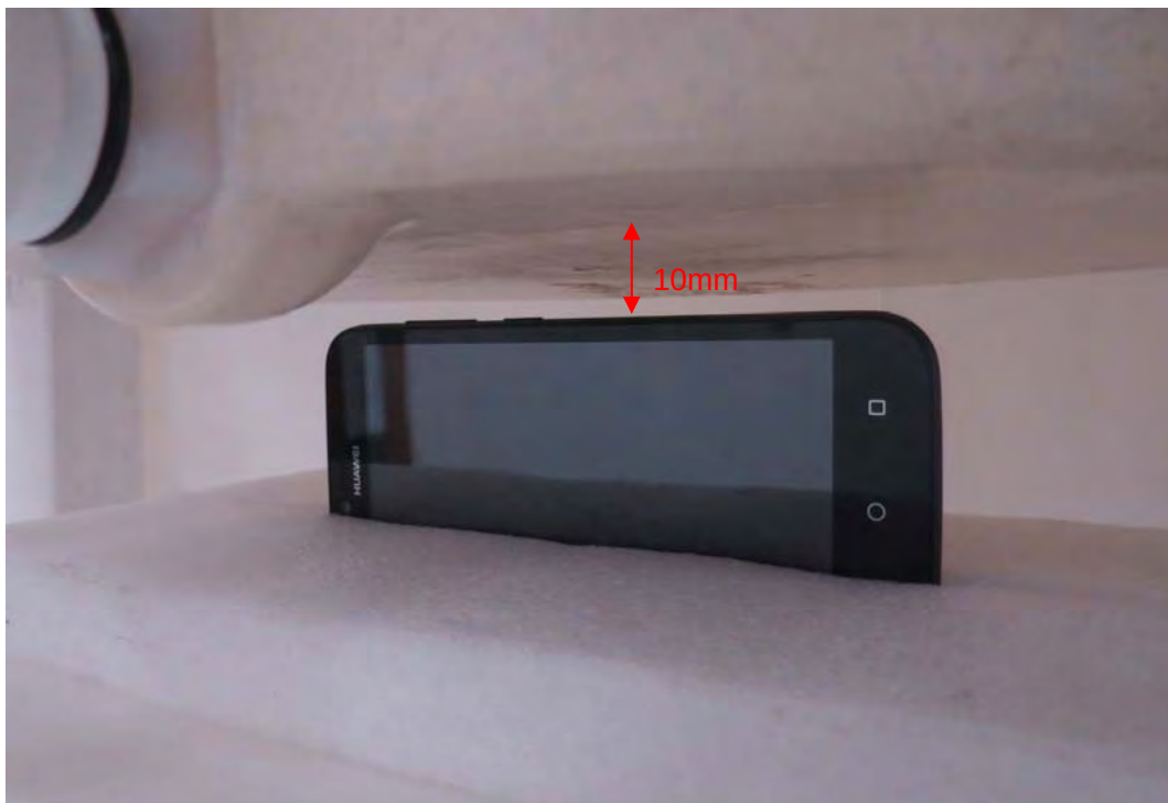
Picture 16: Right Edge, the distance from handset to the bottom of the Phantom is 10mm
