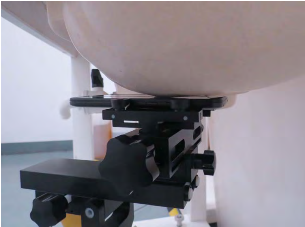
Picture 9: Left Hand Touch Cheek Position
