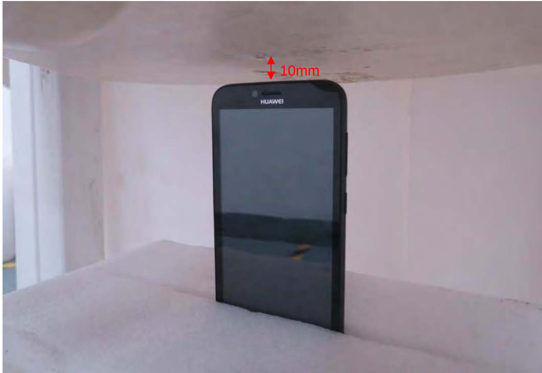
Picture 17: Top Edge, the distance from handset to the bottom of the Phantom is 10mm (Original Model)
