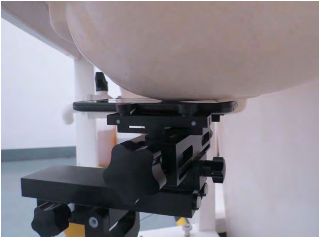
Picture 9: Left Hand Touch Cheek Position (Original Model)
