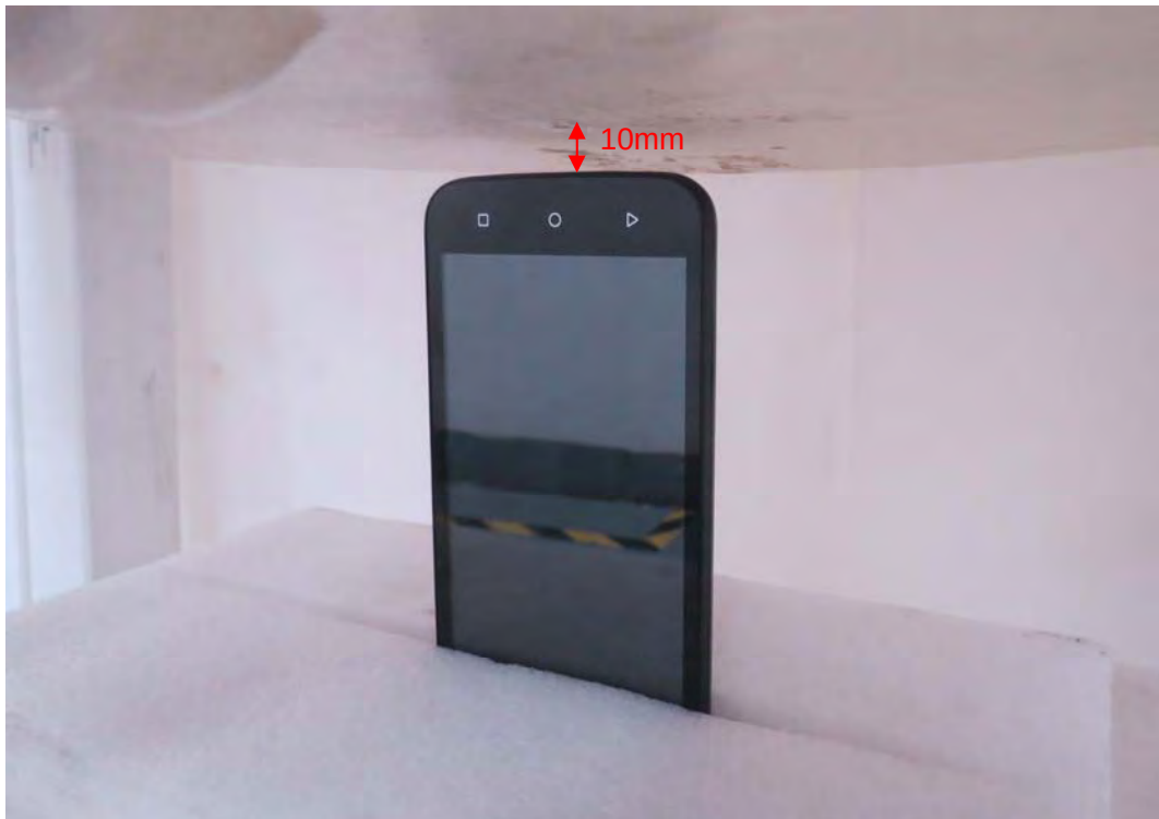
Picture 18: Bottom Edge, the distance from handset to the bottom of the Phantom is 10mm (Original Model)
