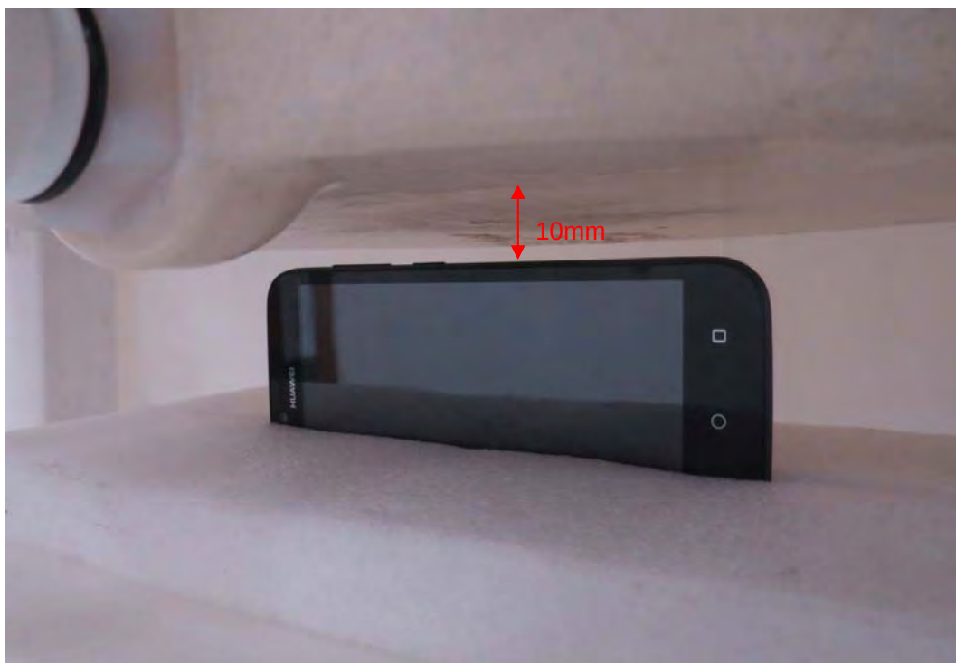
Picture 16: Right Edge, the distance from handset to the bottom of the Phantom is 10mm (Original Model)
