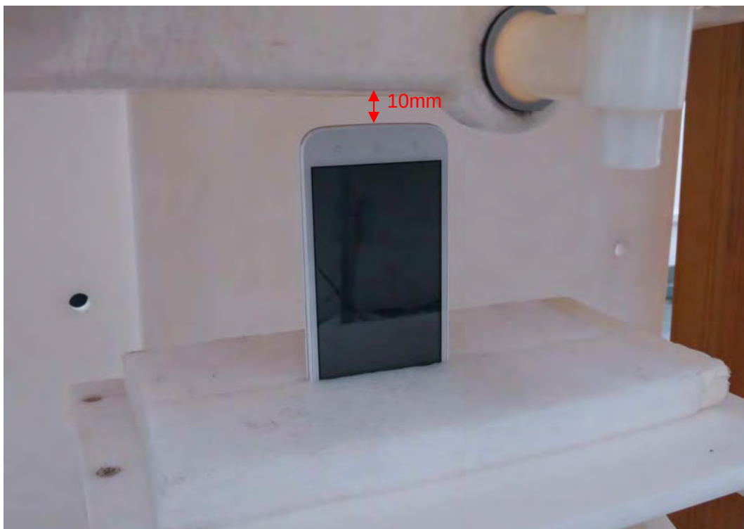
Picture 22: Bottom Edge, the distance from handset to the bottom of the Phantom is 10mm (Variant Model)
