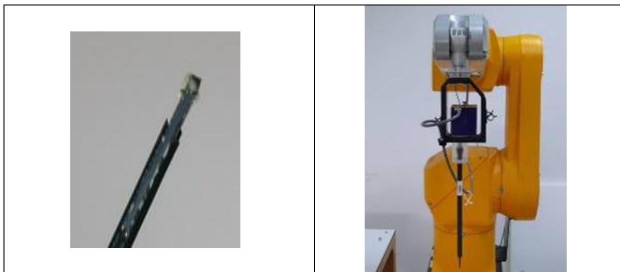
EX3DV4 E-field Probe
