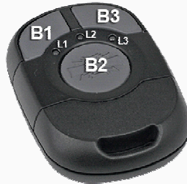
Figure 5: Keyfob control with allocated Buttons and LEDs names
