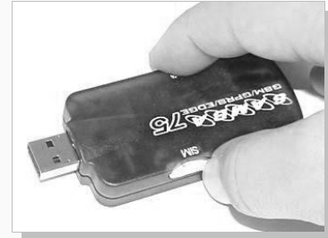
Figure 6: Push it forward into the SIM-Card reader.
