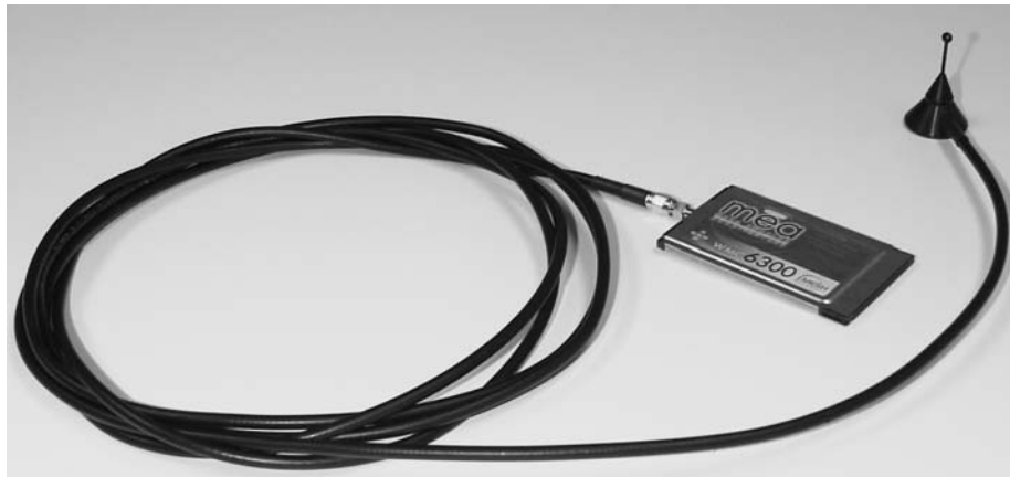
Figure 10. Attach Magnetic Mount Antenna to the WMC6300
