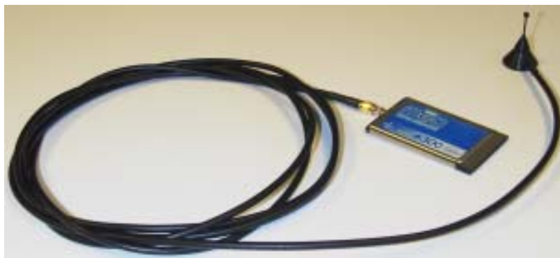
Figure 14. Attach Magnetic Mount Antenna to the WMC6300
