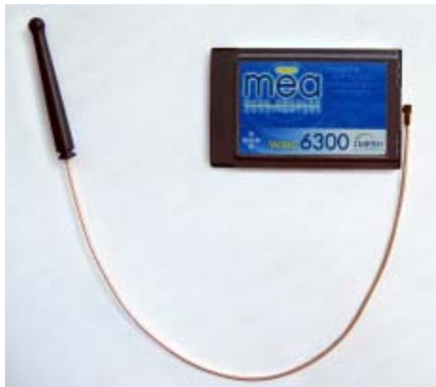
Figure 10. Attach Antenna to the WMC6300
