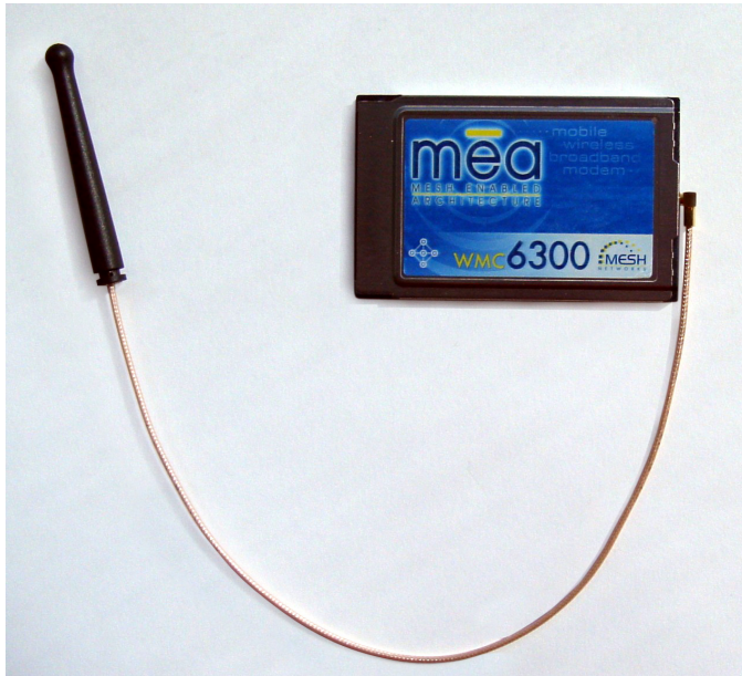
Figure 10. Attach Antenna to the WMC6300
