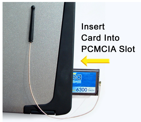
Figure 15. Installing the WMC6300 Wireless Modem Card
