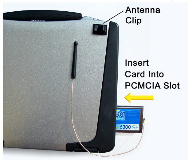
Figure 12. Mounting the Antenna Clip
