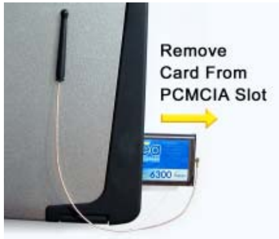
Figure 18. Removing the WMC6300 from the PCMCIA slot
