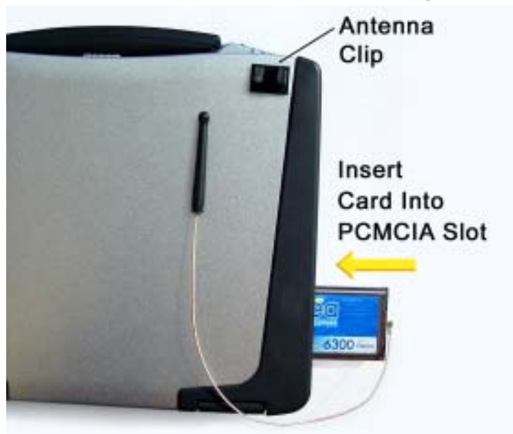
Figure 13. Mounting the Antenna Clip
