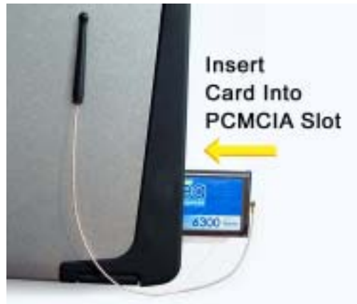
Figure 16. Installing the WMC6300 Wireless Modem Card
