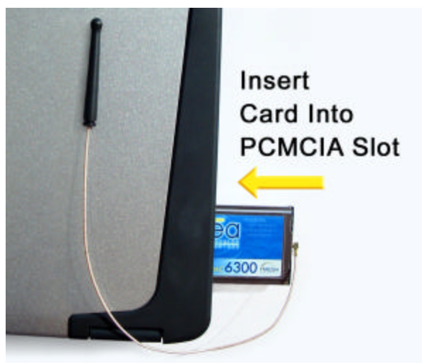
Figure 25. Installing the WMC6300 Wireless Modem Card
