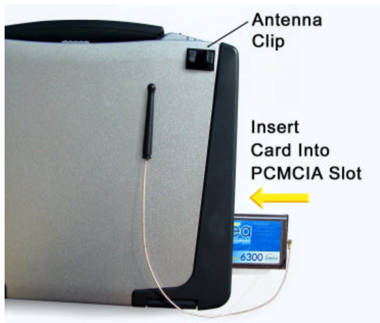
Figure 22. Mounting the Antenna Clip
