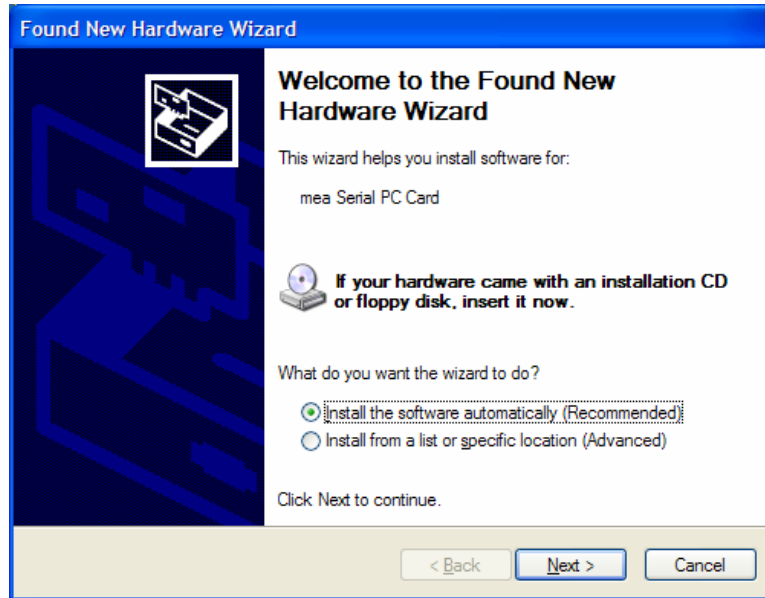
Figure 3-6 Found New Hardware Wizard – Serial PC Card
