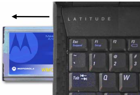
Figure 3-17 Removing the WMC6300 from the PCMCIA slot
