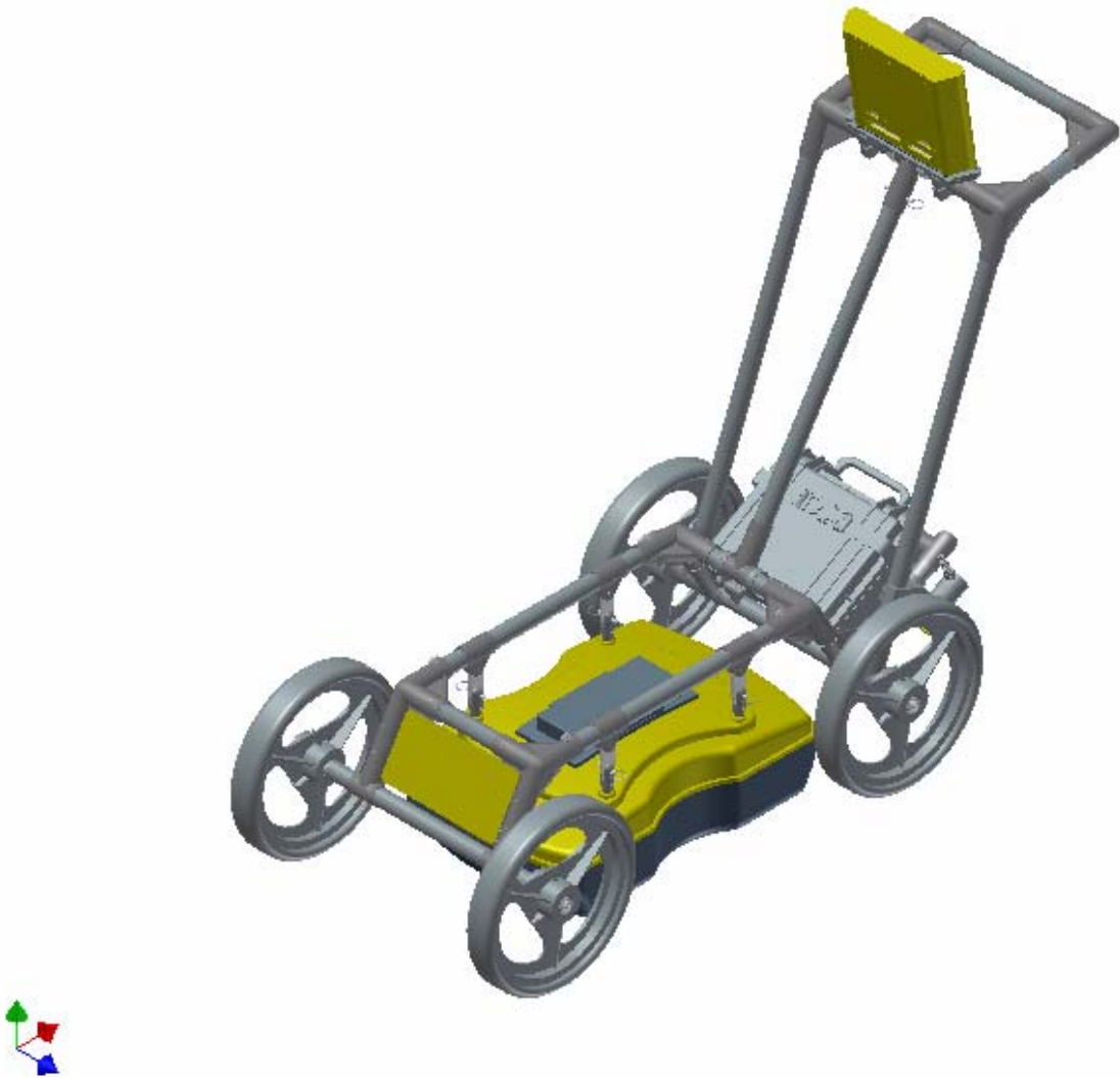
Figure 2-1: Fully assembled Smart Cart
