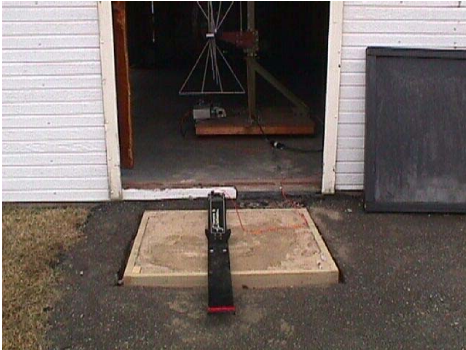
Test Configuration #3: Pulse Ekko Pro with 50 MHz Antenna
