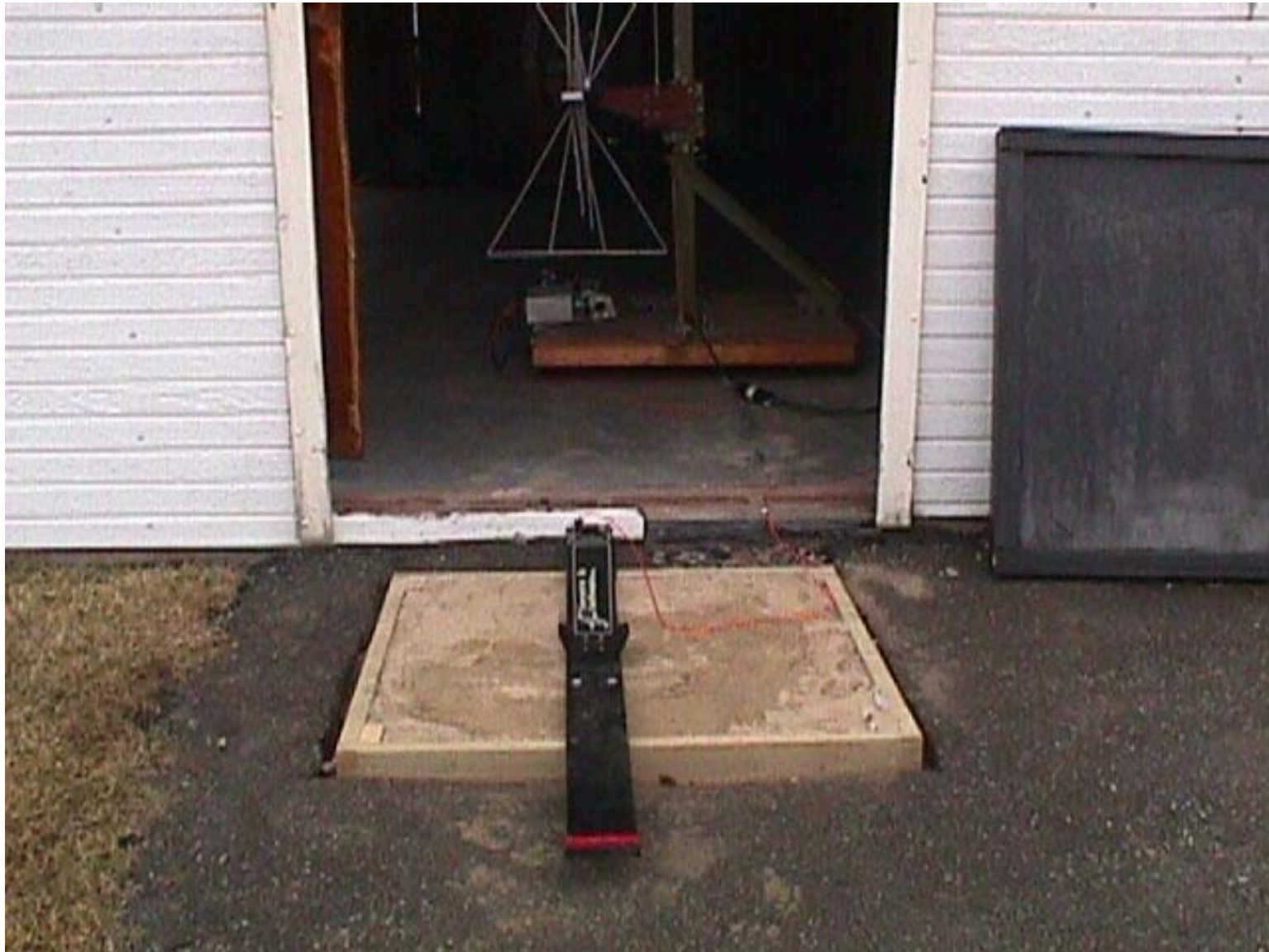
Test Configuration #3: Pulse Ekko 100 with 50 MHz Antenna
