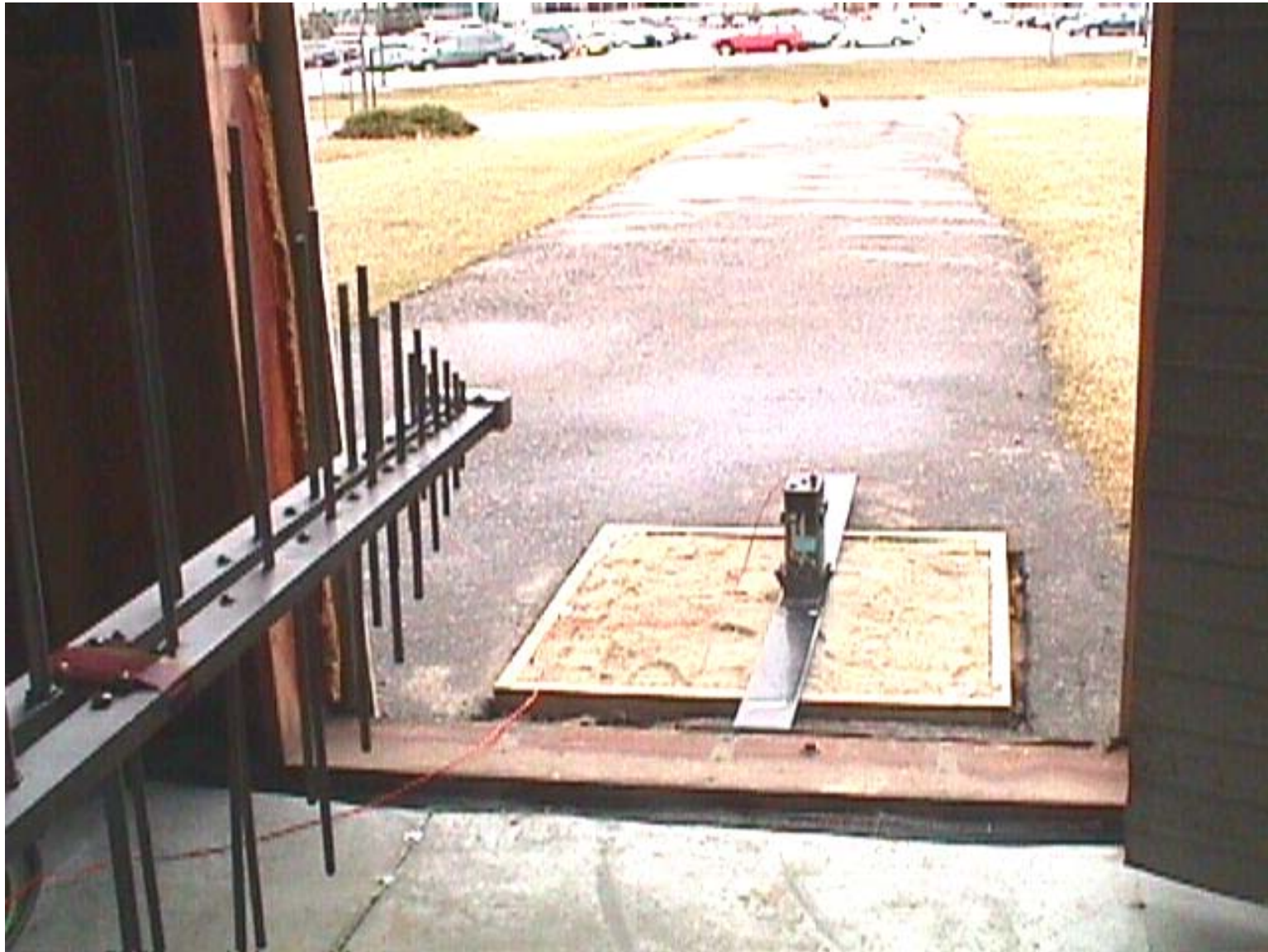
Test Configuration #3: Pulse Ekko 100 with 50 MHz Antenna
