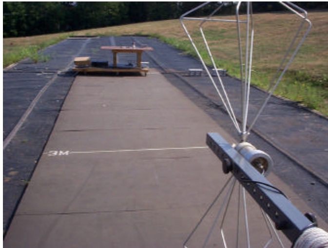
Biconical antenna Frequency range 30-200MHz
