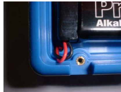
Figure 5. INCORRECT battery connector lead
