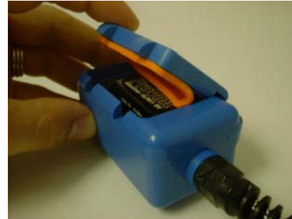
Figure 3. INCORRECT gasket seating
