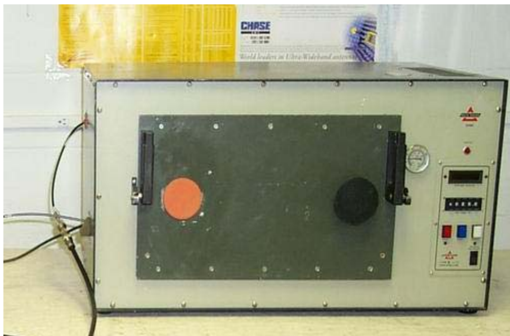
Figure 3.3 Frequency Tolerance Test Setup ( Tx device only)
