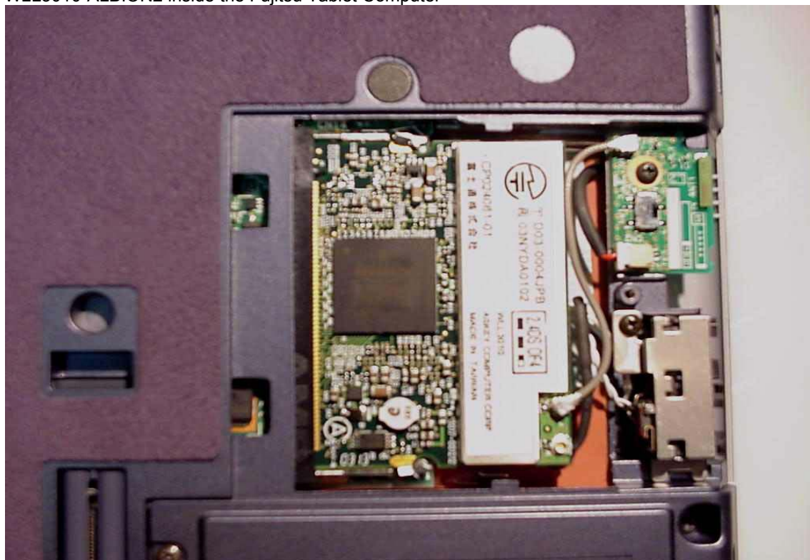
WLL3010-ALBION2 inside the Fujitsu Tablet Computer
