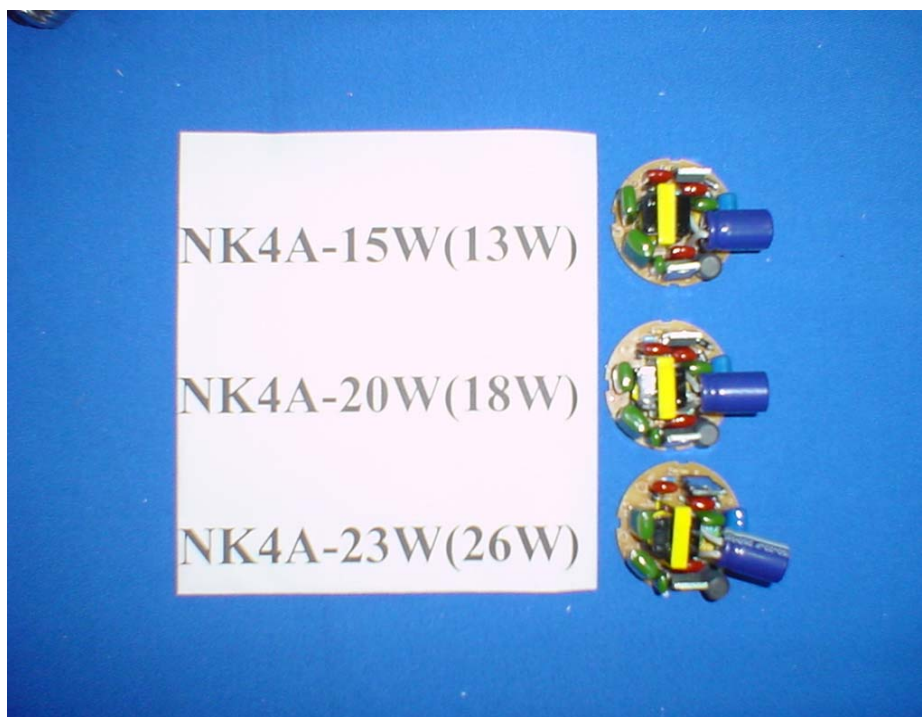
Figure 5 M/N: NK4A Series Main Board, Component Side
