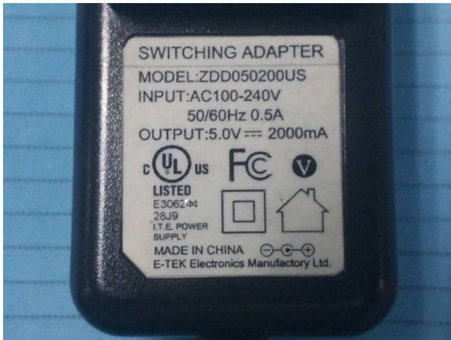
EUT – Adapter Label View
