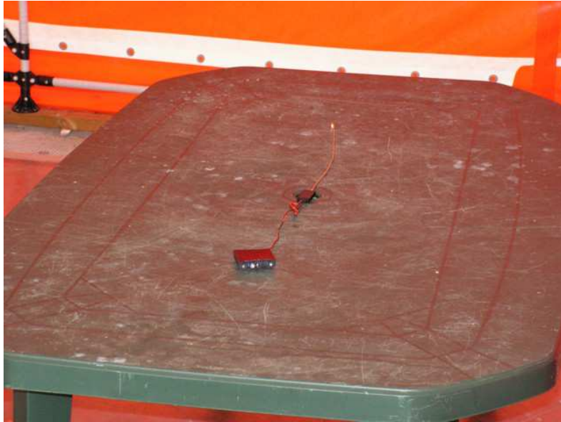
TXFH-RC field strength set up for max radiation
