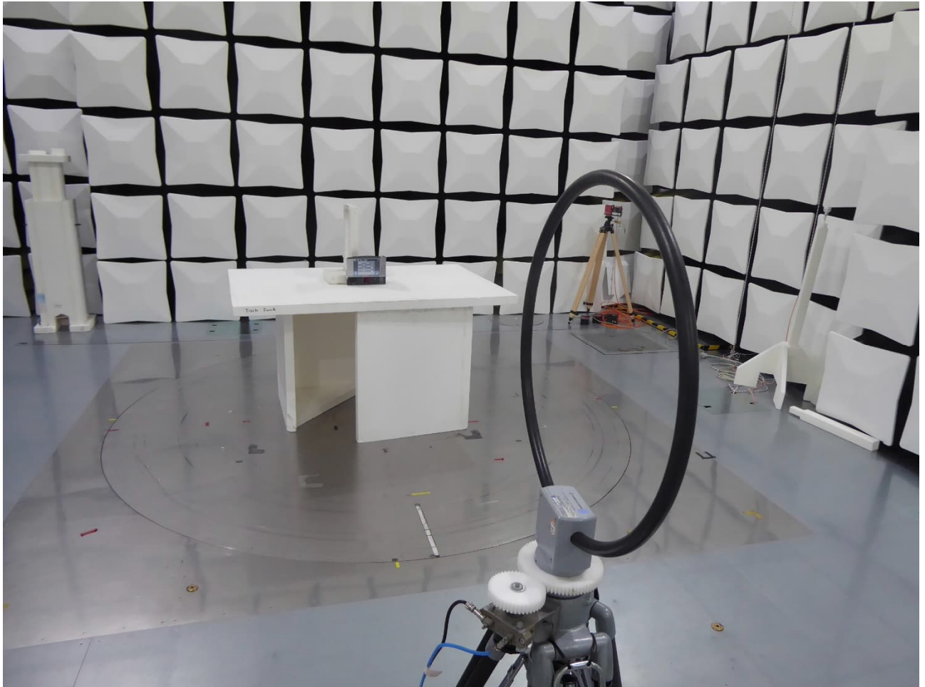
9 kHz – 30 MHz - antenna position 2
