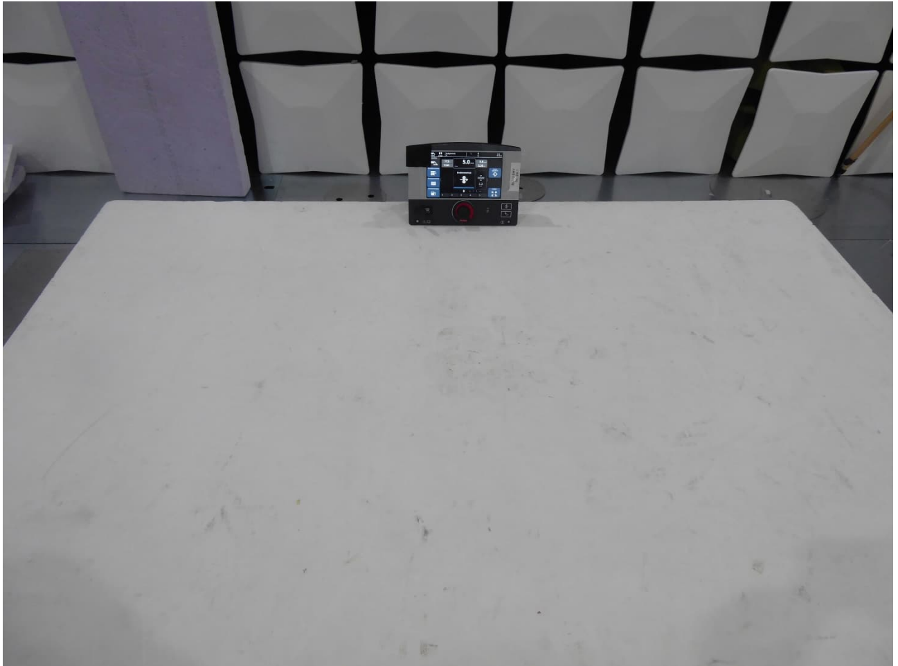
EUT Setup – radiated emissions
