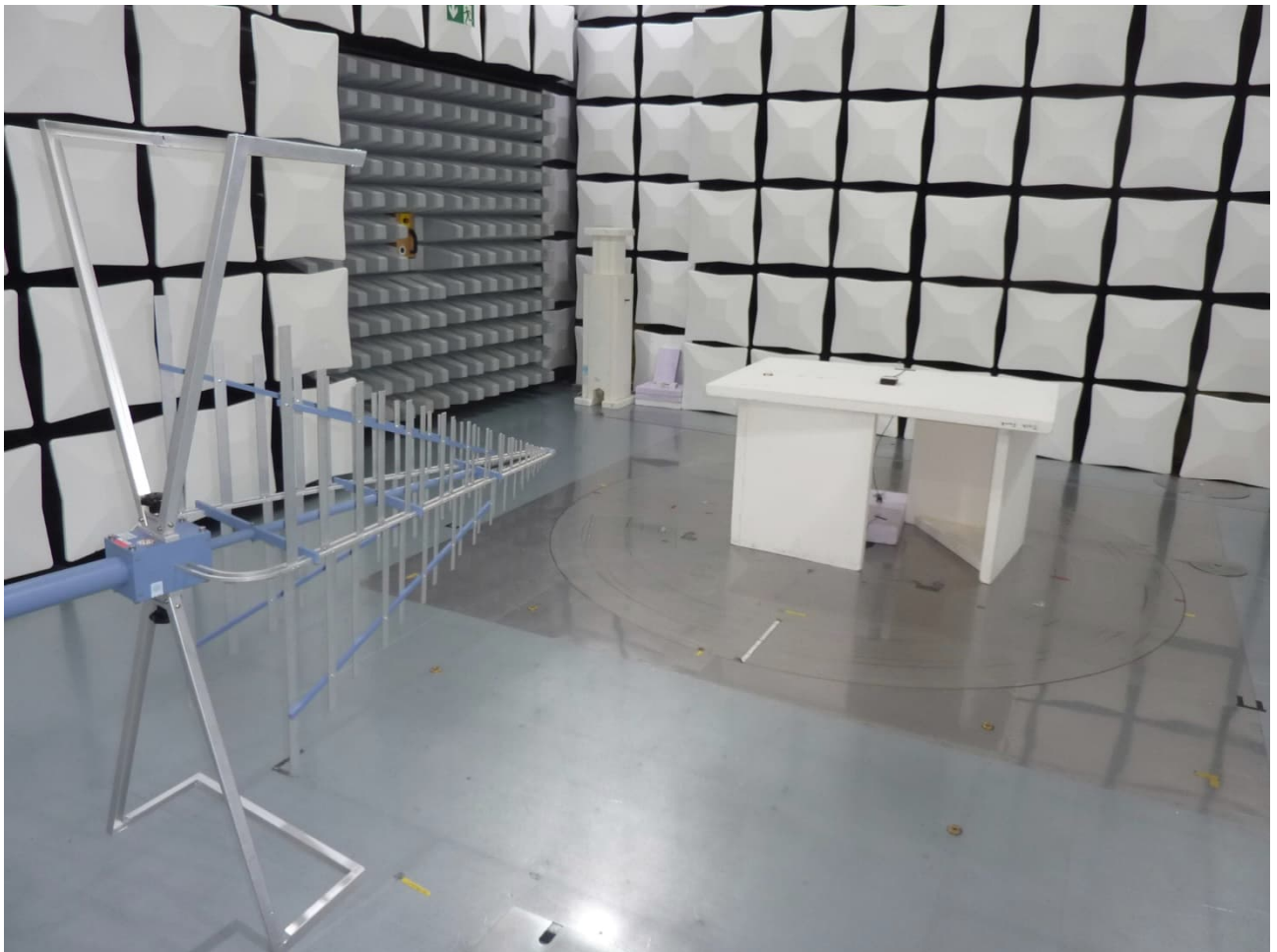
Test setup semi anechoic chamber <1 GHz
