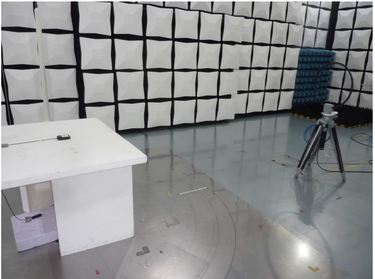
Test setup semi anechoic chamber <30 MHz
