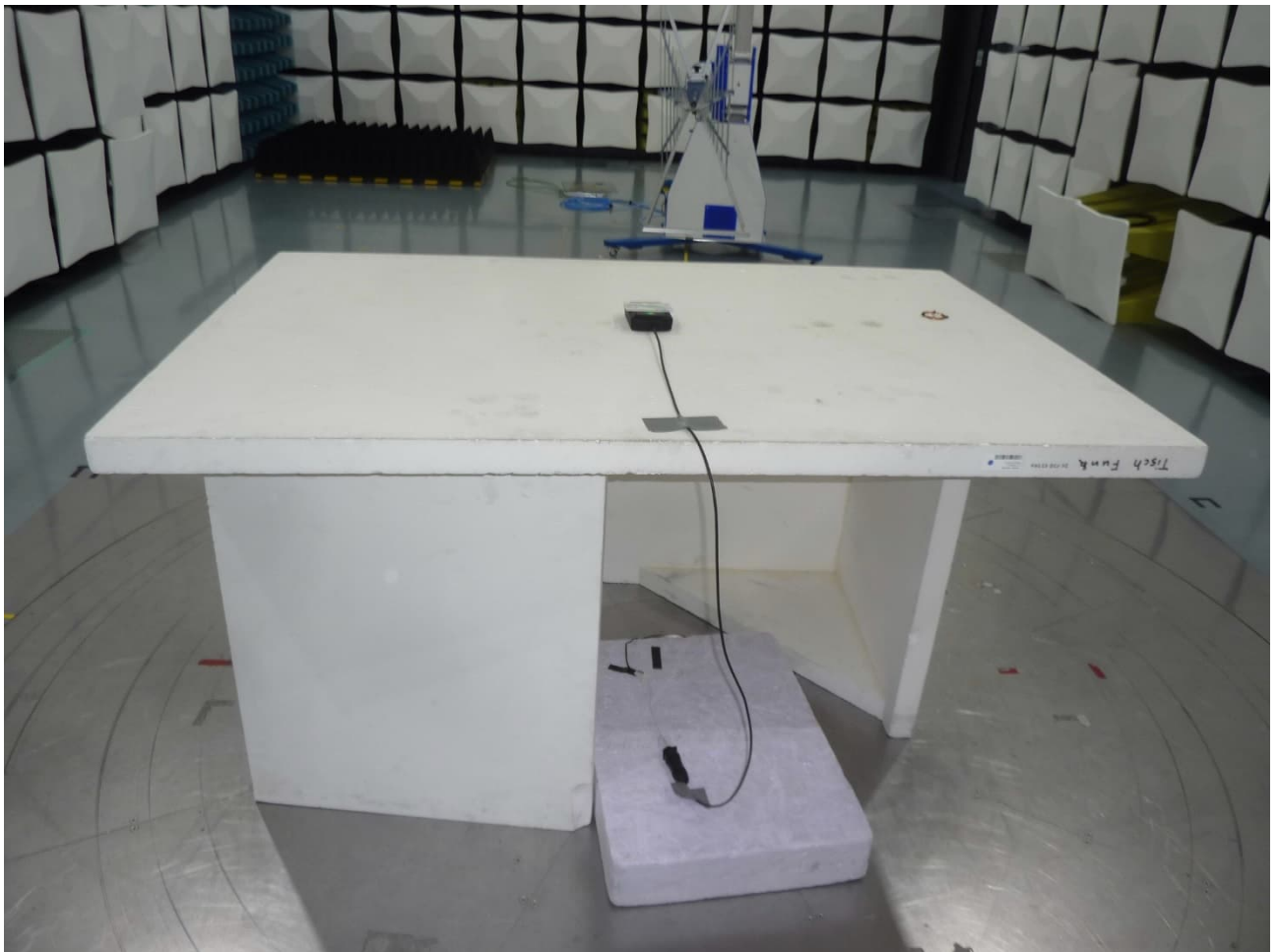
Test setup semi anechoic chamber <1 GHz
