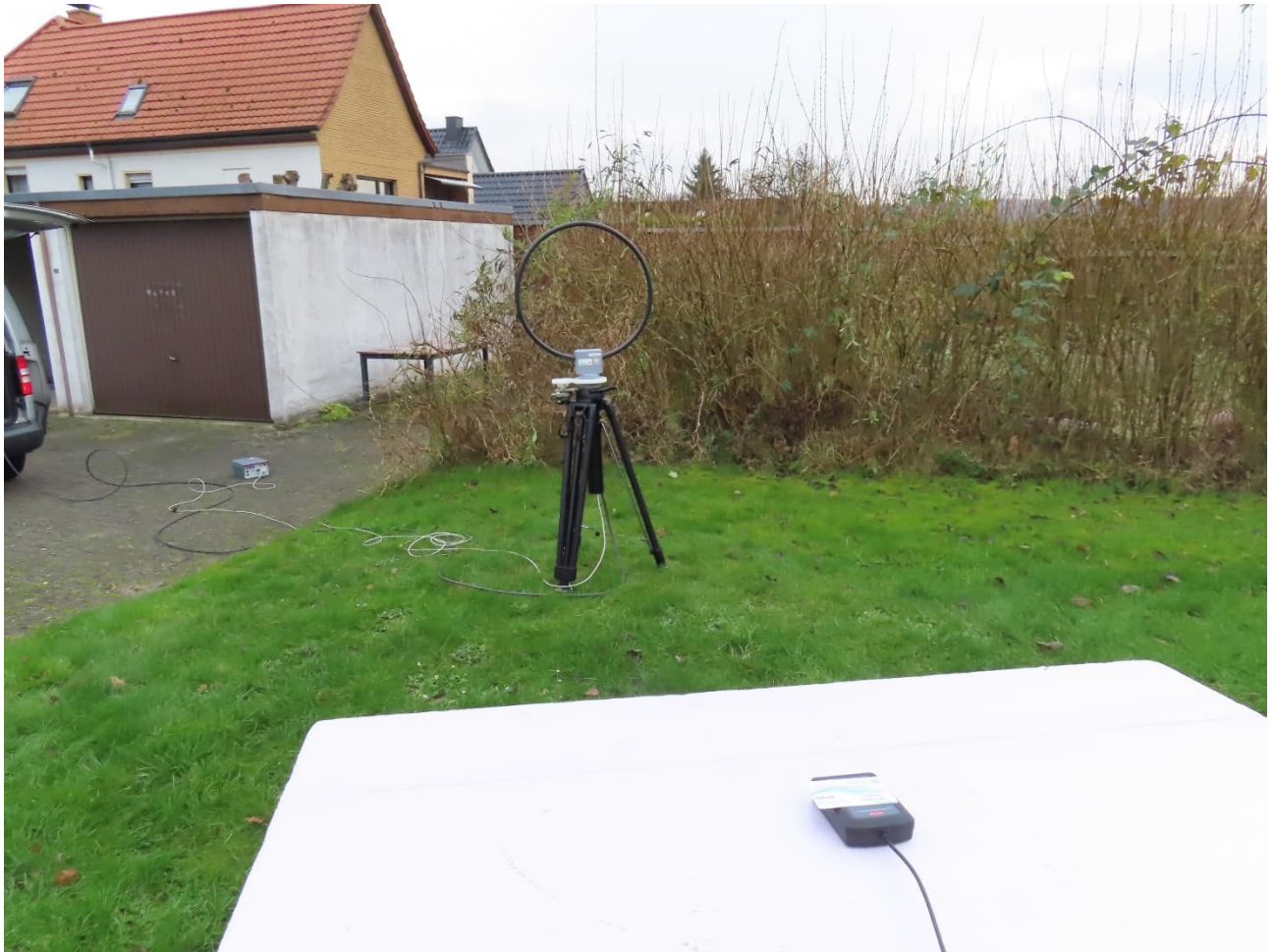
Test setup outdoor test side <30 MHz
