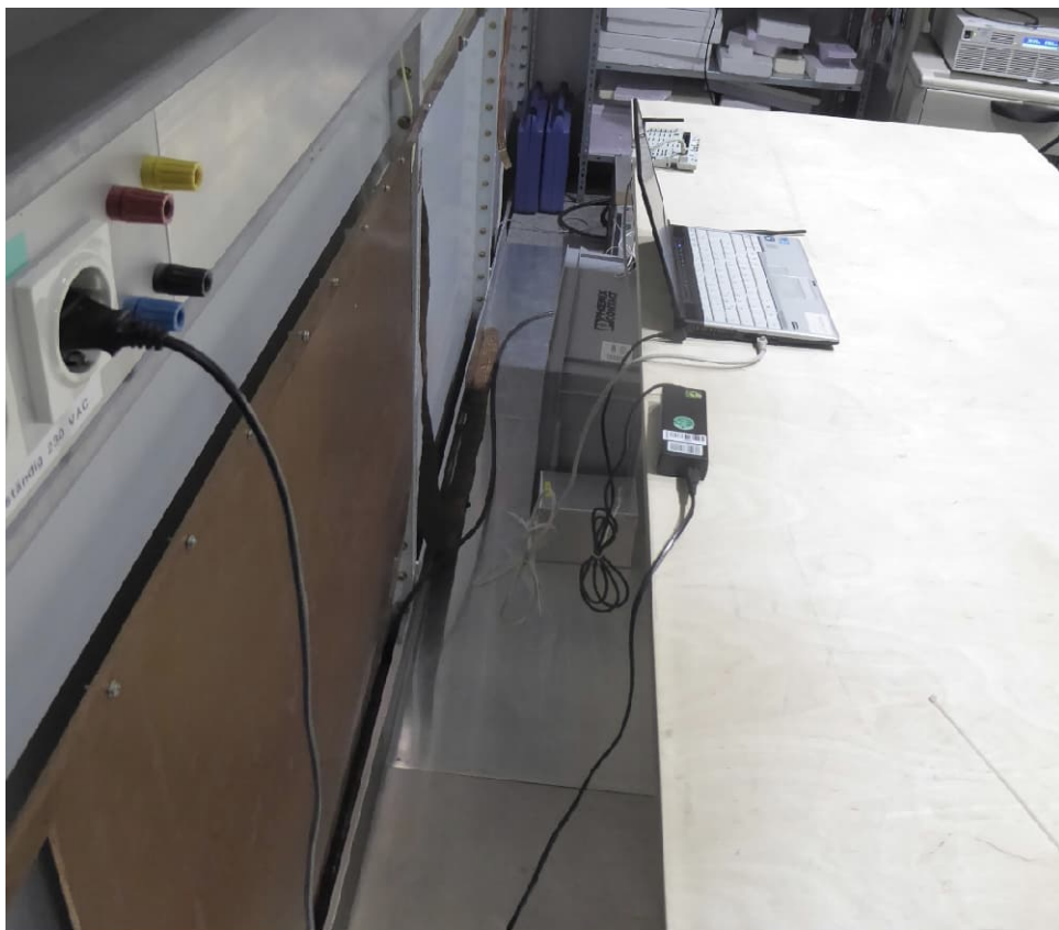
AC powerline conducted measurement
