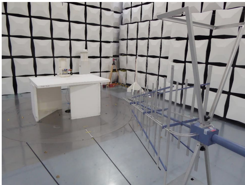
Test setup semi-anechoic chamber M276 Preliminary and final measurement
