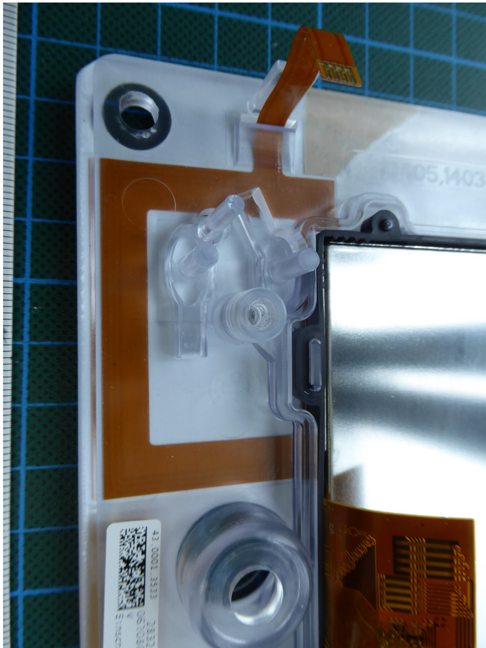
Detail view to loop antenna
