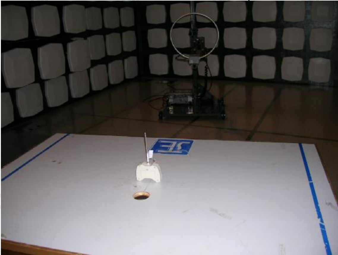
Measurement of Radiated Emission Test Set Up
