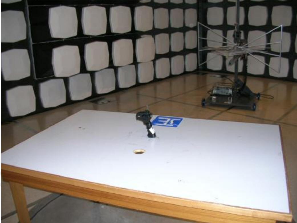
Measurement of Radiated Emission Test Set Up
