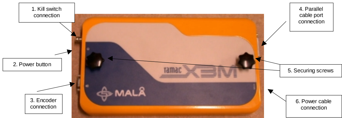
Figure 2.1a. Layout of the X3M
