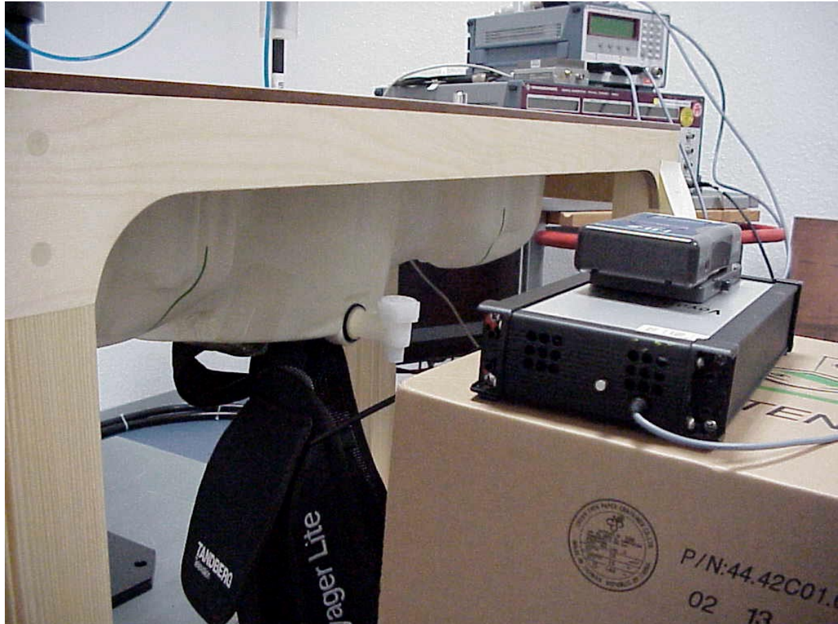
Photo 2: Patch antennas against the body phantom
