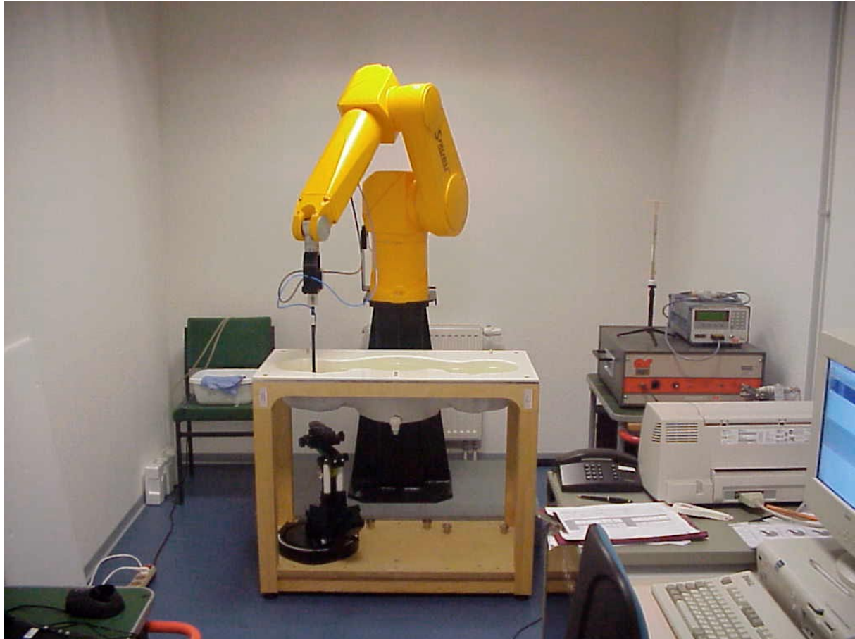
Photo 1: Measurement System DASY 3
